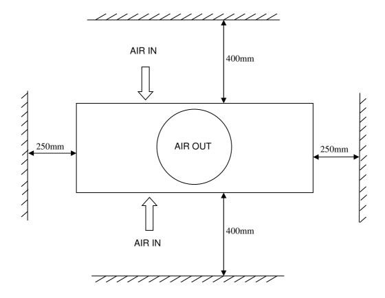
A gap of at least 1000mm is required above the dehumidifier.
